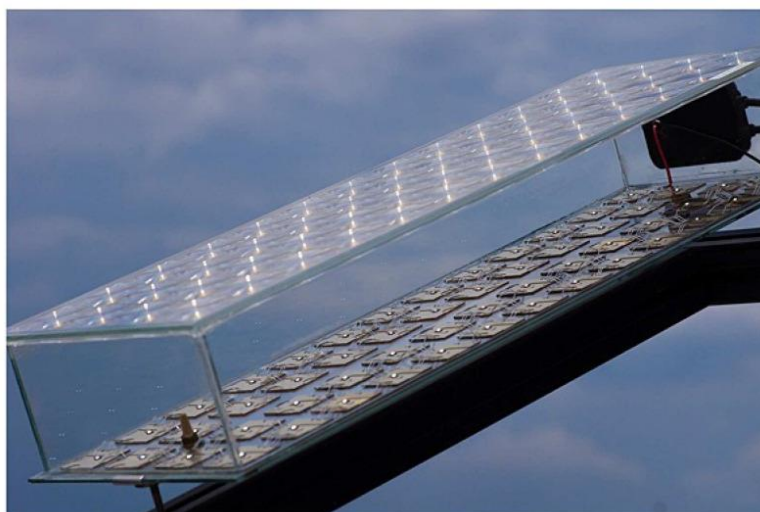
Figure 3-33 FLATCON® CPV module with 52 four-junction solar cells (see [RD22])
